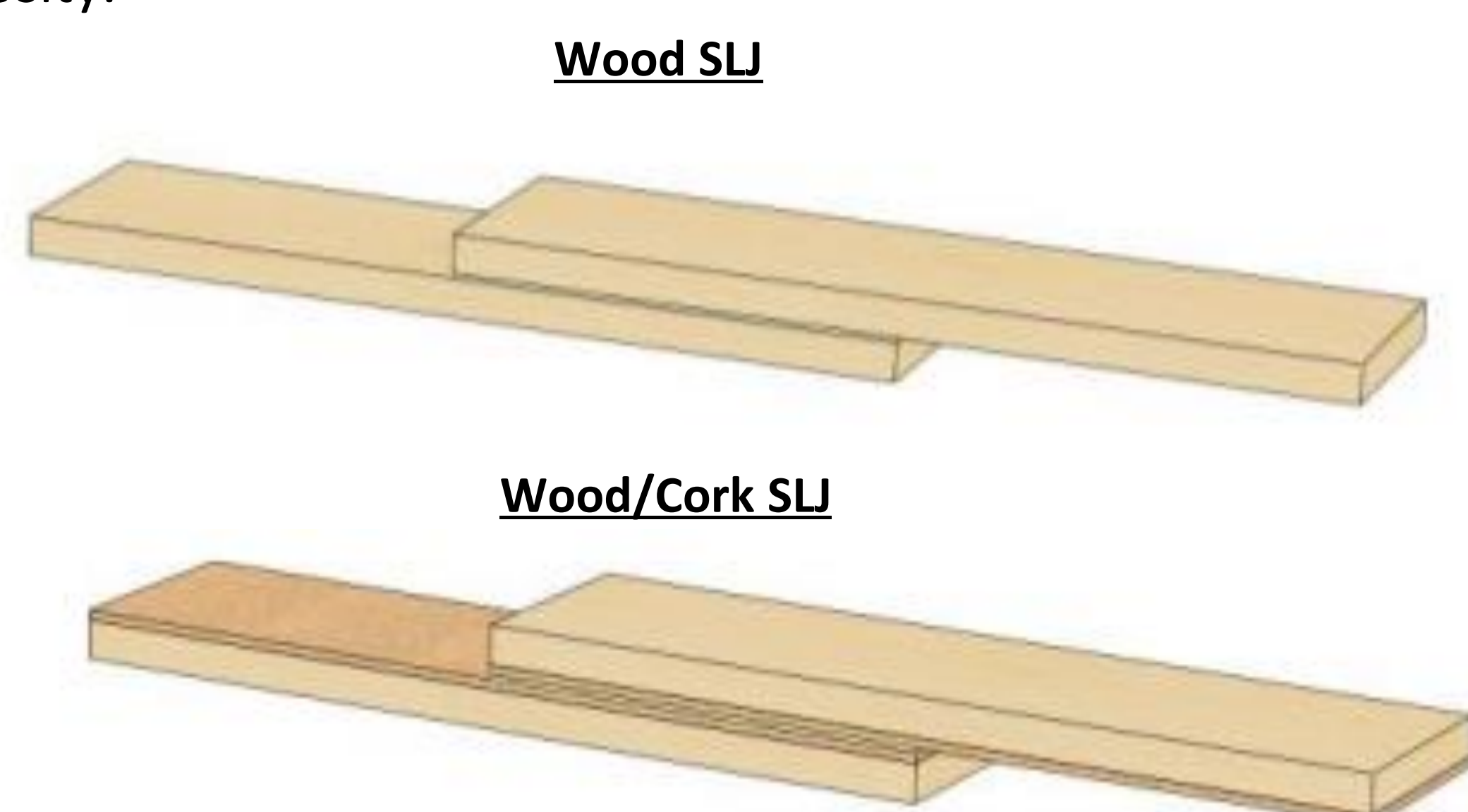
FIGURE 2. SLJ specimen configurations.
